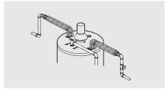
Typical horizontal piping arrangement
